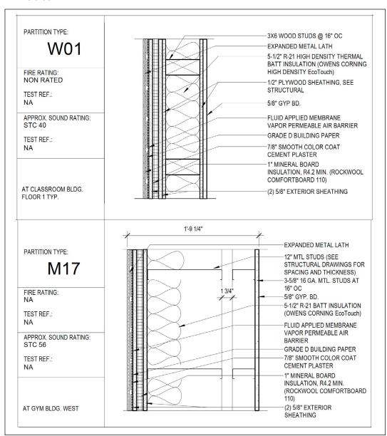
(Right) Wall details called out in the wall sections on the opposite page. Detail W01 uses 2X6 wood studs. Detail M17 uses 12" metal studs for structural reasons. (Courtesy of Ratcliff Architects)
