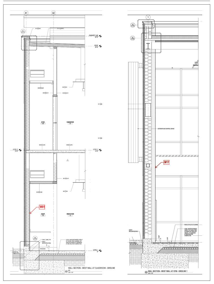
The concrete floors are uninsulated. The roofs generally are insulated with 5"-thick rigid cellular polyisocyanurate sheets. The gymnasium roof, constructed of steel decking, is sloped to drain and is covered with uniform rigid insulating sheets having an overall U-value of 0.036. The class-room building roof consists of standard wood framing with tapered sheets of insulation to provide the necessary drainage and has an overall average U-value of 0.032.
