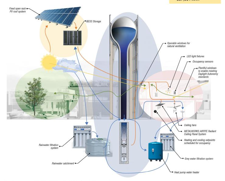
**Heating System** - METALWORKS AIRTITE Radiant Ceiling Panel System, Water Source Heat Pump, Mechanical heat exhaust exchange from Hydroelectric Turbines .
