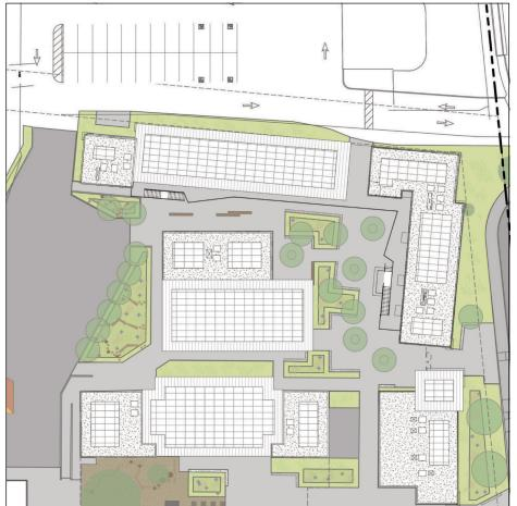
(Top Left) Roof plan of Ocean View ES from the 2023 Solar PV Feasibility Study showing solar panels installed on new building roofs and a new car canopy.
