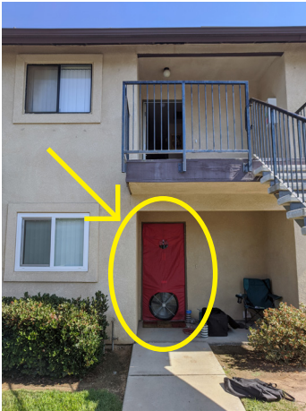
(Above) Blower Door test in place at Building 619, Vera Cruz Village.
