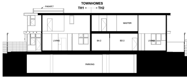
TRANSVERSE (CROSS) SECTION @ TOWNHOMES - LOOKING NORTH
