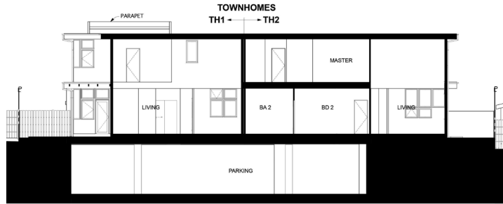
TRANSVERSE (CROSS) SECTION @ TOWNHOMES - LOOKING NORTH
